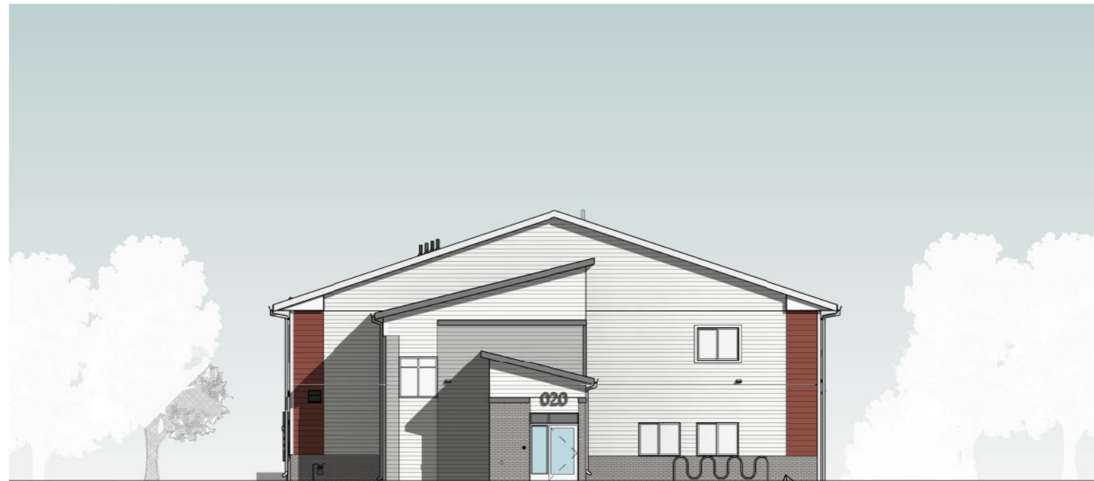
2 NORTH ELEVATION - WEST BIRCH APARTMENTS 1/16" = 1'-0"
