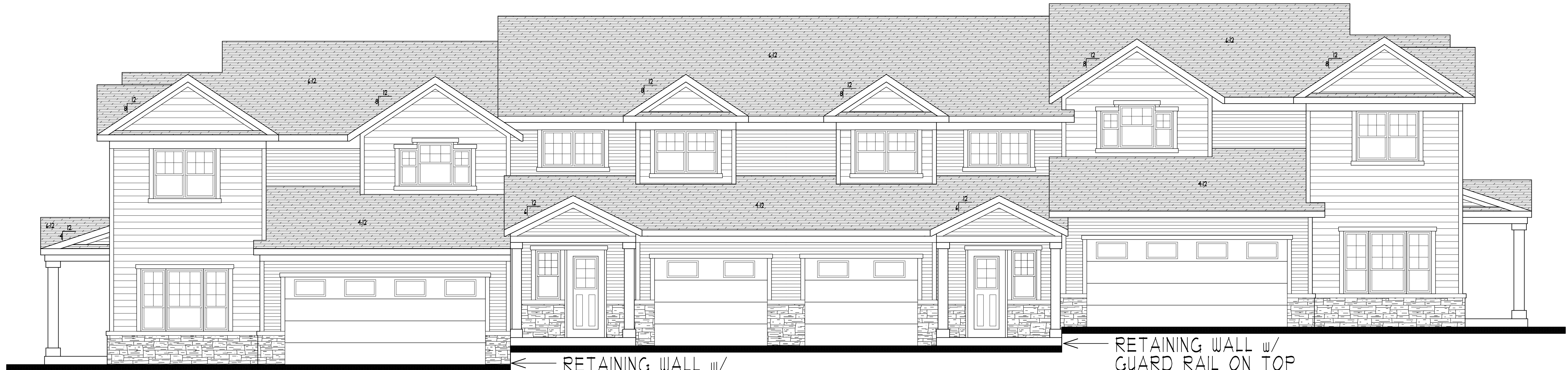
FRONT ELEVATION - BLDG. "4-2" SCALE: 1/4" = 1'-0"
