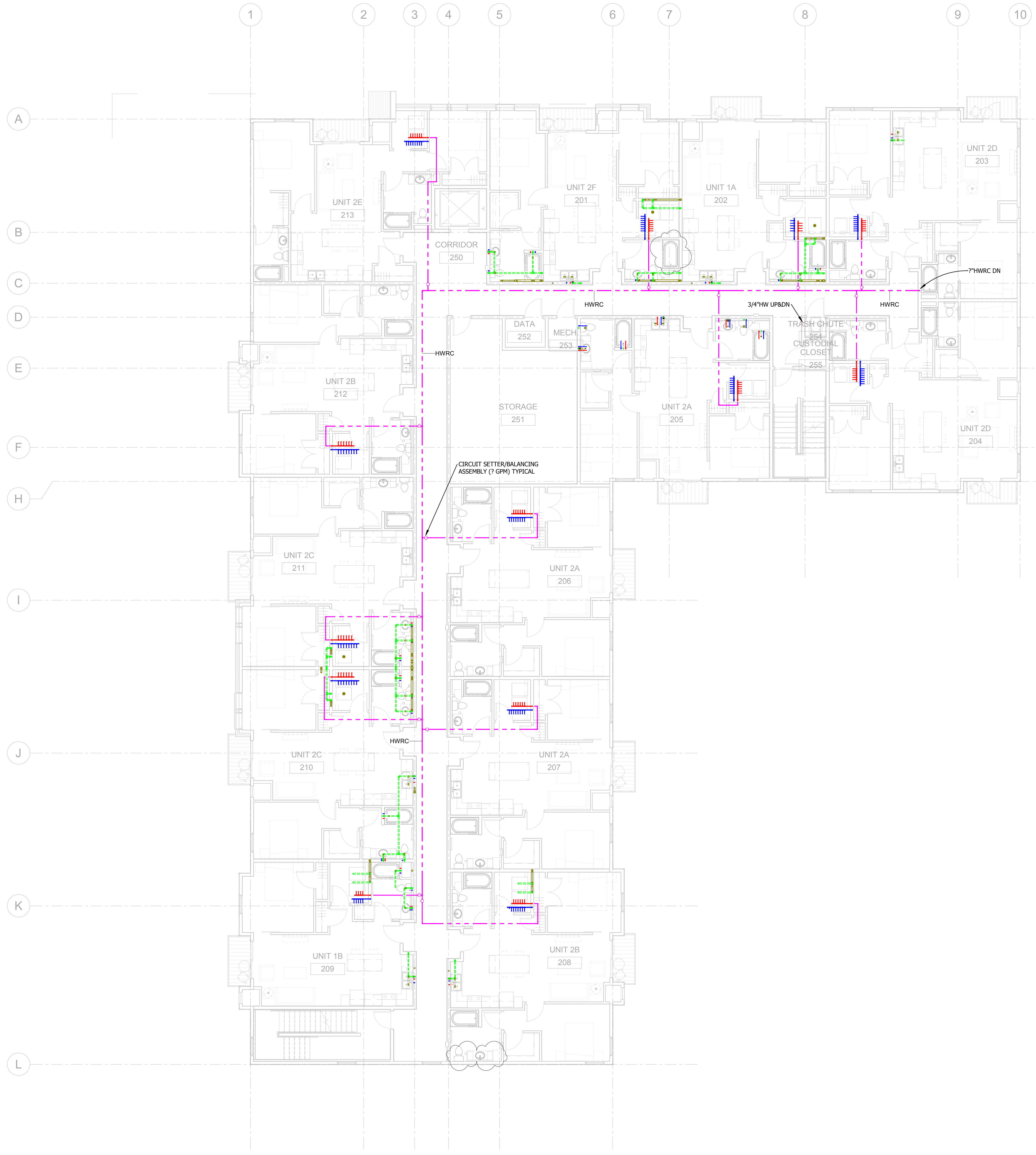
1 SECOND FLOOR - PLUMBING PLAN 0 4' 8' 16'
